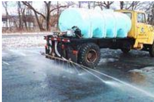
District 5's Tanker and Spray-bar system
