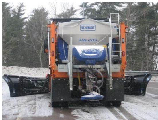
The Schmidt Stratos slide-in “V” hopper spreader
