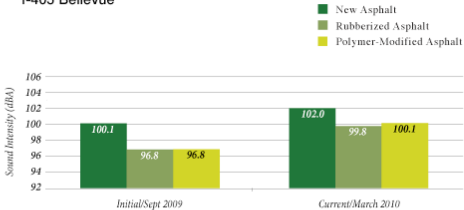
Figure 2.28: I-405 Initial and Current OBSI Noise Measurements.
